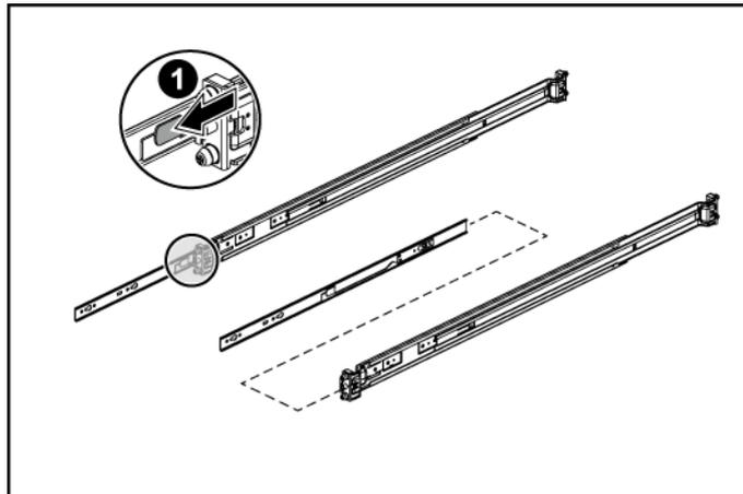
2. Align the inner rail to the retaining posts on the side of the switch.
