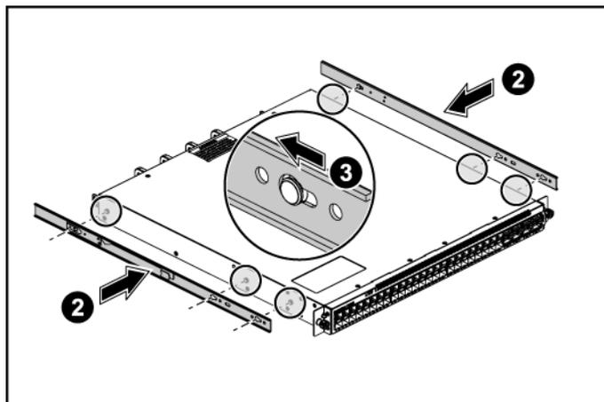
4. Press the retaining clip on the rear end as indicated.
