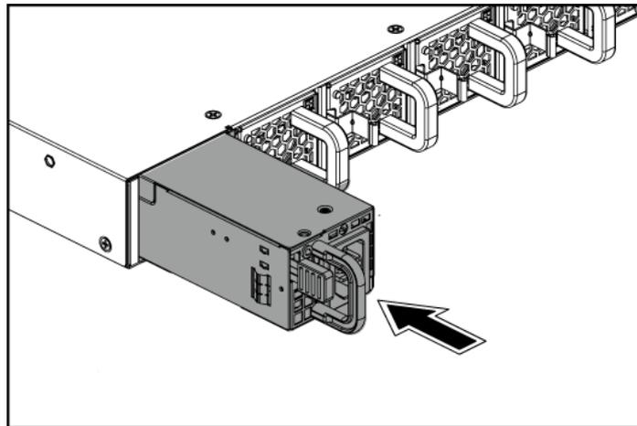
The AC power connector is a standard three-pronged connector. The switch automatically adjusts its power setting to any supply voltage in the range from 100-240 VAC at 50-60 Hz.
