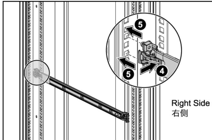
6. Press the retaining clip on the front end as indicated.
