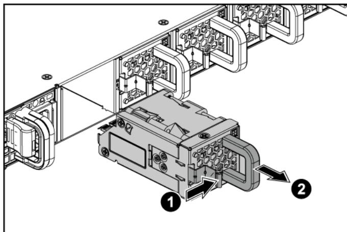
3. Push the system fan module into the system fan module bay until it connects properly with the fan board in the chassis.
