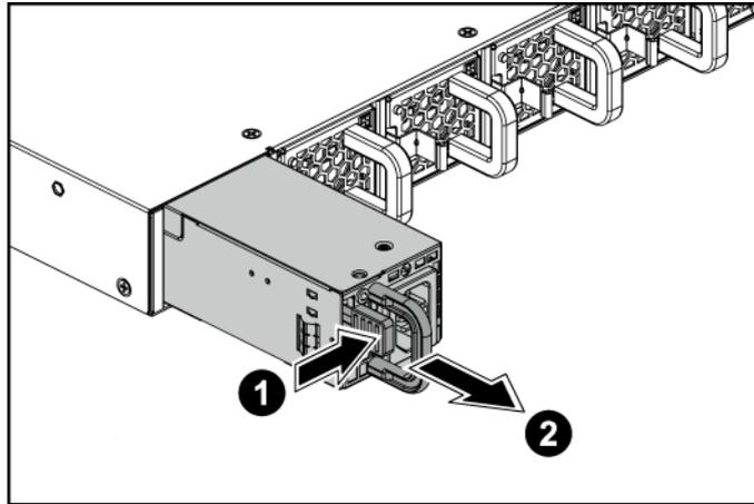
3. Align the PSU with the switch bay.
