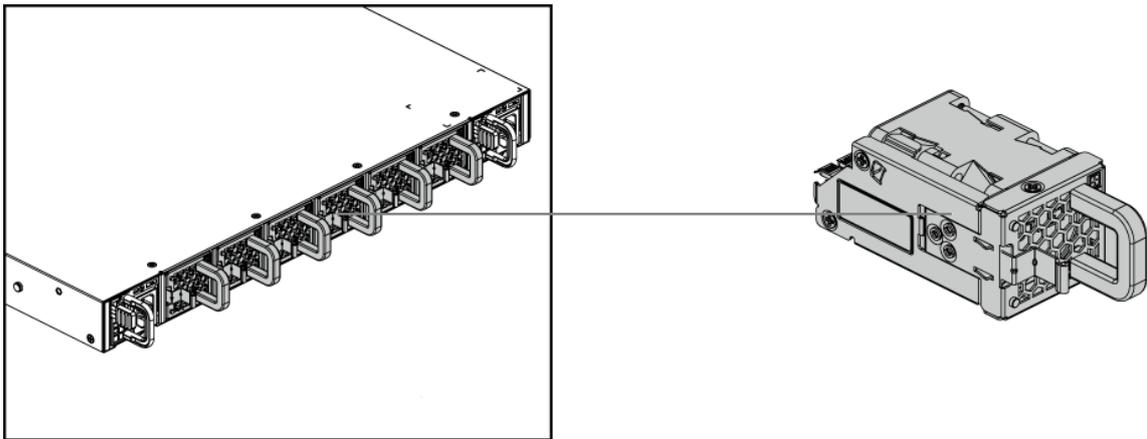
The fan module is a field replaceable unit and can be replaced during operations as long as the remaining modules are installed and operating.
