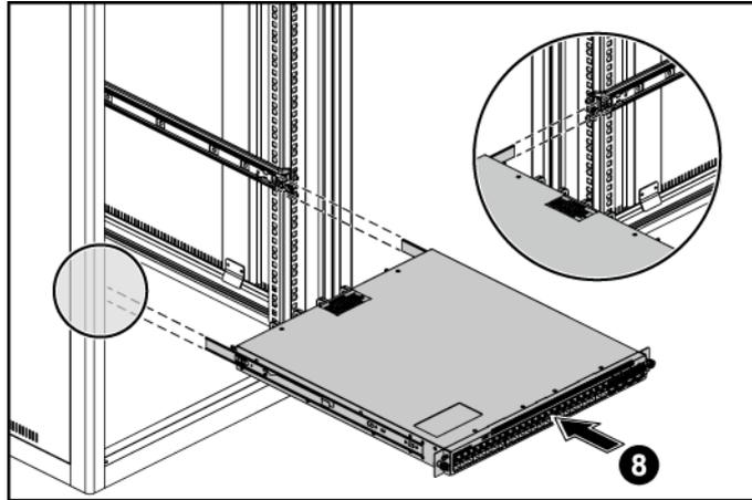
9. Tighten screws on both sides to lock switch on the rack.
